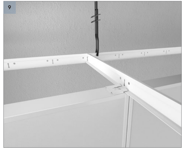
Two baffles suspended at a slot of T24 ECR profiles. Use the dimples on the sides of the baffles to align perfectly.
