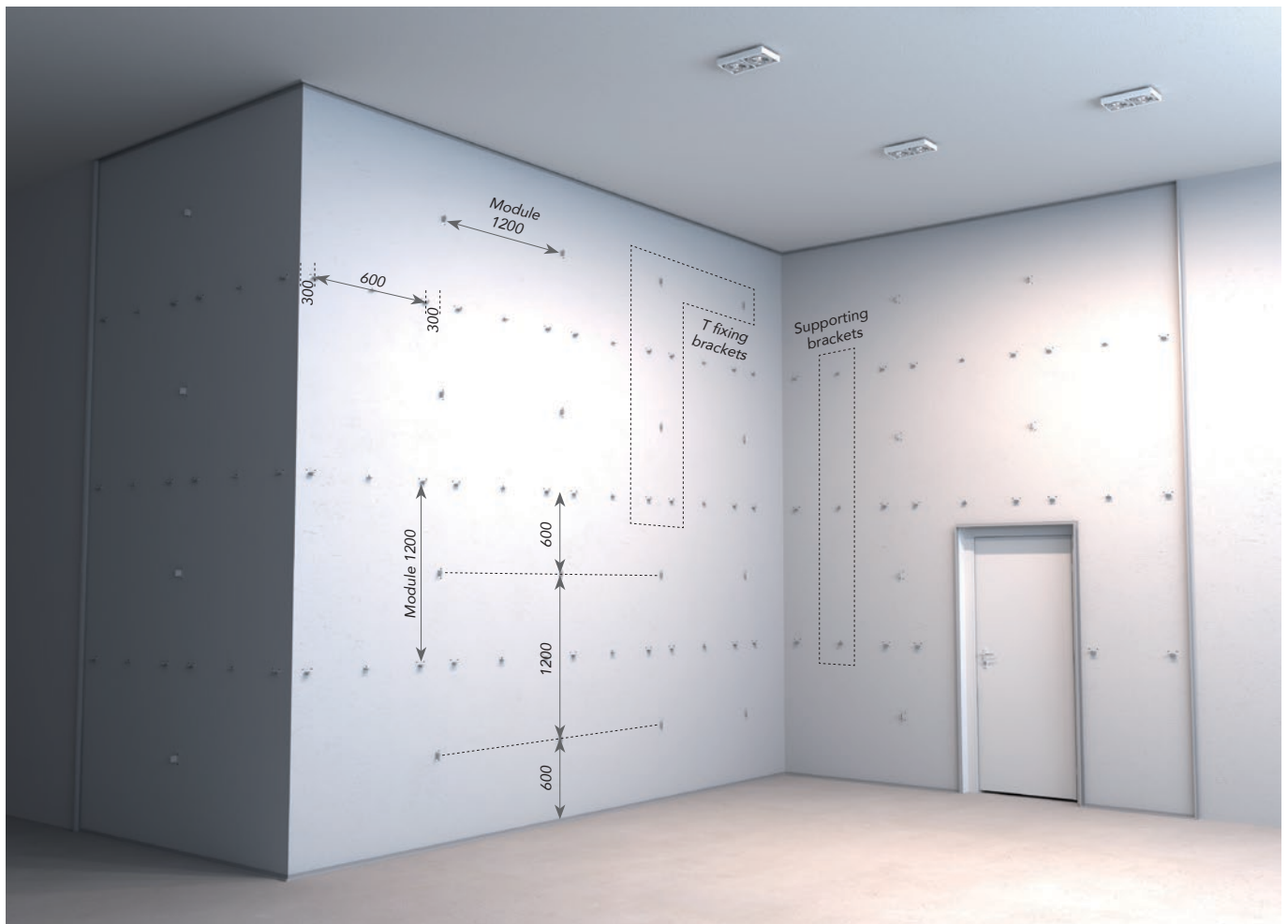
2.1 Placement of all T fixing brackets and supporting brackets should be measured out and mounted before any panel installation begins. Doing so will greatly reduce installation time. Ensure that all brackets line up – T fixing brackets' channel on the module axis, supporting brackets' underside 4 mm above it.
