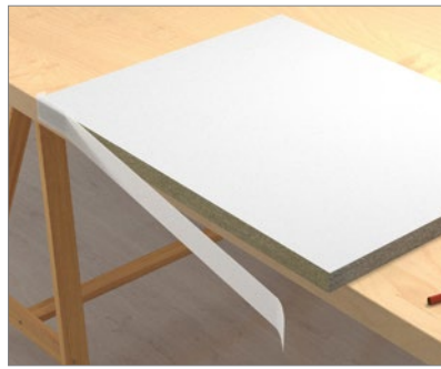
3. Align 5 mm overlap on front and press.
